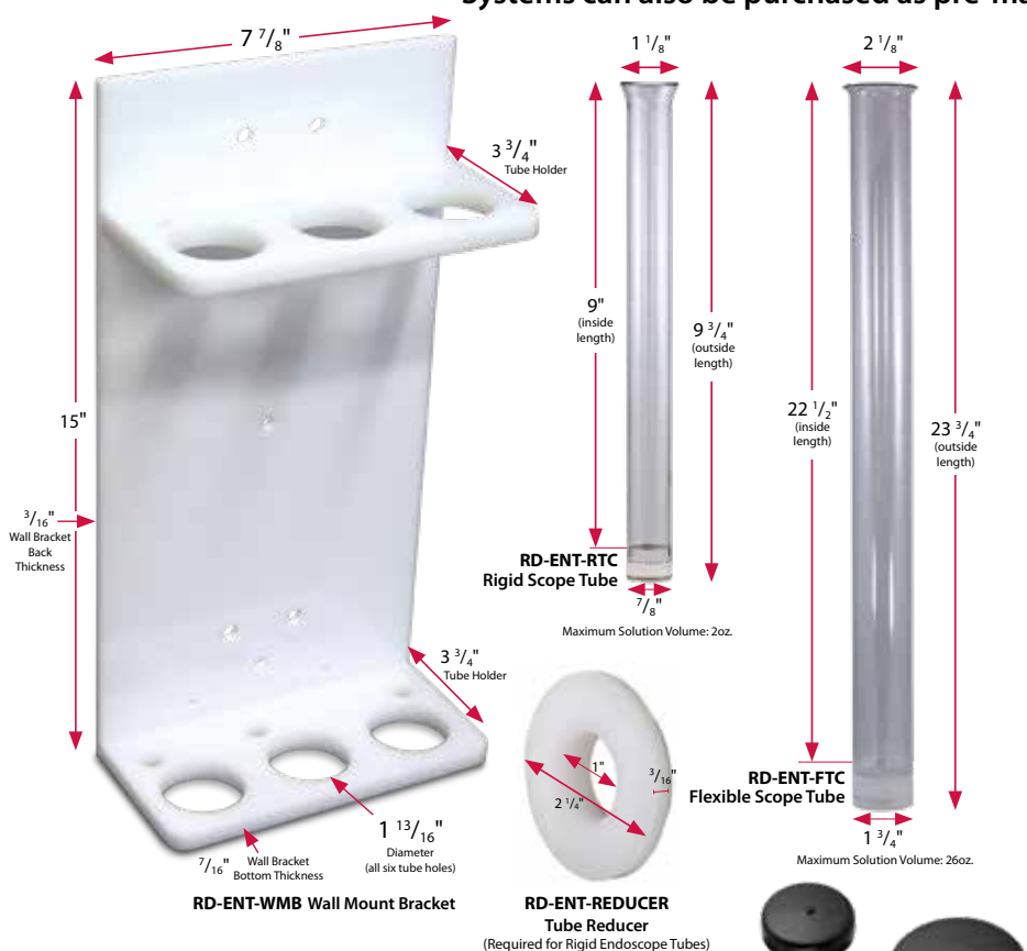
Universal Wall Bracket accommodates BOTH Flexible and Rigid Endoscope Tubes
