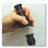
2. Connect the magnification lens to the endoscope eyepiece using the c-clamp.
