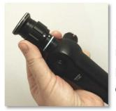
1. Ensure your endoscope is in focus. Often there are markings on the endoscope focus ring indicating a neutral position. Ensure your light source is connected and power is on.
