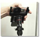
6. Insert the magnification lens with attached endoscope into the c-clamp on the adaptor platform.
