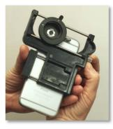
5. Turn over the adaptor platform and use the threaded screw to line up the viewing hole with the smartphone camera lens. Use your thumbs to align the camera lens in the opposite axis.
