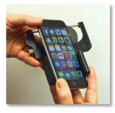
4. Place the edge of a smart phone into the spring-loaded clamps on the adaptor platform and use thumbs to snap into place.
