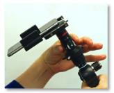
8. Adjust focus ring on magnification lens or refocus endoscope to perfect image quality.
