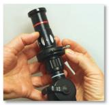
3. Ensure the lens c-clamp is held flush and firm against the endoscope eyepiece, then tighten the locking screw so the lens is stable and secure.
