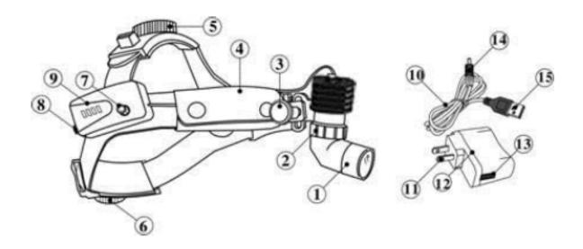
1.Light holder 2.Light spot adjusting ring 3.Lock switch of the Light head 4.Headband 5.Top tightness-adjusting knob 6.Back tightness-adjusting knob 7.Power switch/brightness-adjusting knob 8.Charging interface of power box 9.Powe box 10.USB wire 11.Internet power plug 12.Charger 13.USB interface 14.Charging plug 15.USB plug
