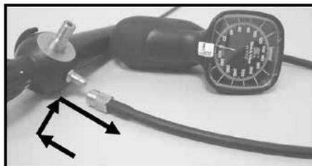
Fig 9. Connection mechanism of leak tester
