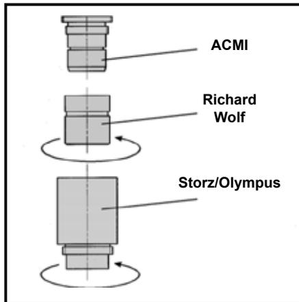
Fig. 6 Fitting the Glass Fiber-optic Connection
